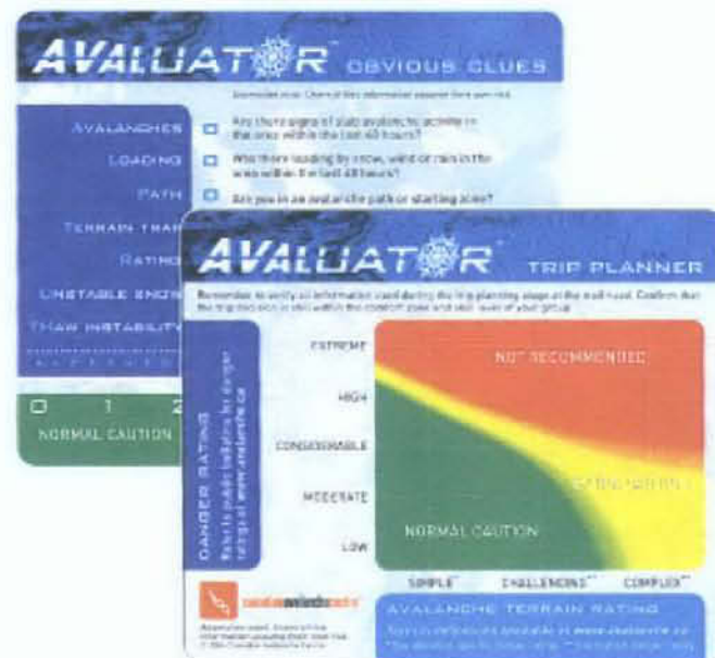
Figure 7. The Avaluator decision support pocket card. On one side, the trip planner uses the ATEs rating and the avalanche danger to inform users of travel recommendations. On the other side a checklist of obvious clues prompts the user to look for danger signs and aids in slope evaluation by making travel recommendations.
