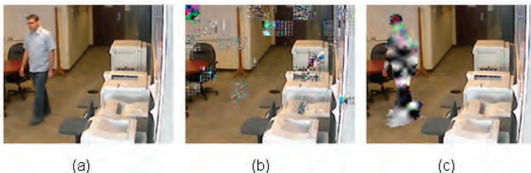
Figure (a): original content stream; Figure (b): both shape and texture have been encrypted and despite attempts to hack into this with an incorrect key, the objects of interest could not be decrypted; Figure (c): example where only the texture of the whole body (or only a face for example) is encrypted.
