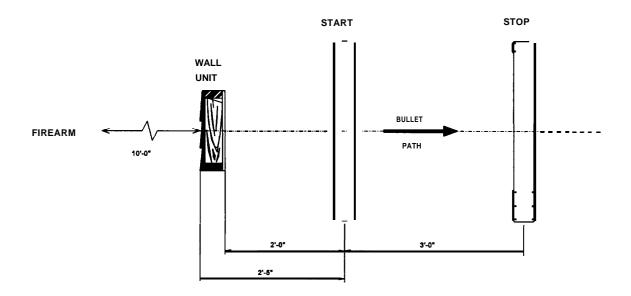
The wall units were screwed to the wood frame while the chronograph screens were bolted to it.
