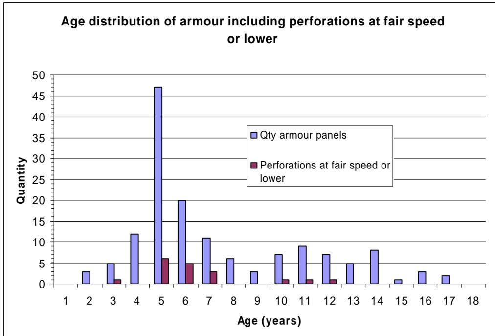
Figure 3: Age distribution of tested armour as well as the fair velocity (or lower) perforations.
