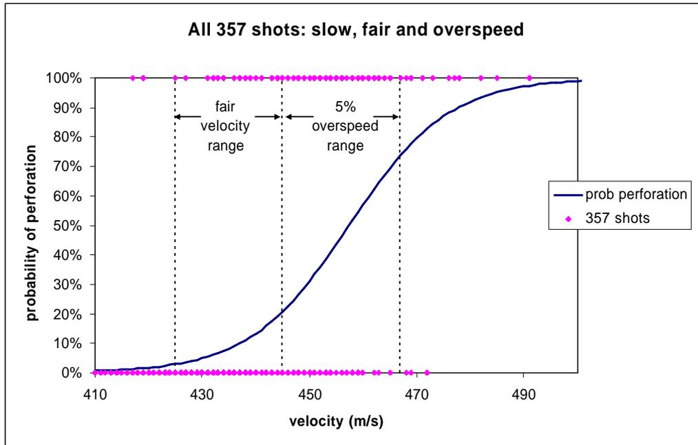
Figure 2: Probability of perforation versus velocity for .357 projectile.
